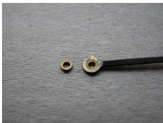
Bush inserted into rod ready for soldering.
