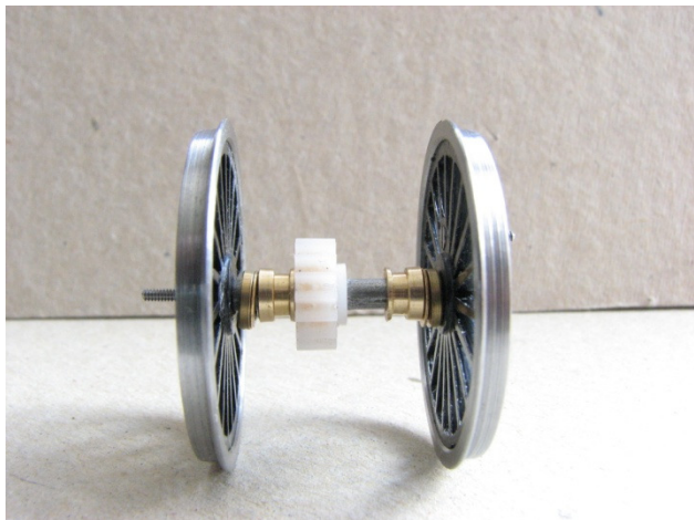
One of the driven axles with spacing washers.
