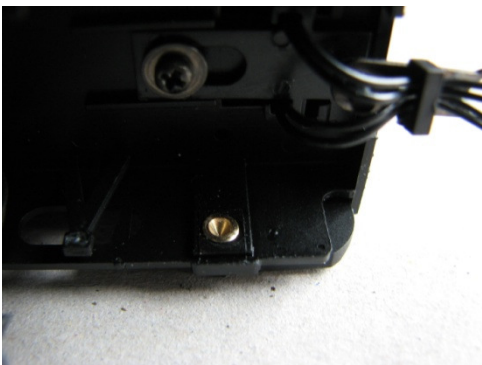
Shouldered pinpoint bearing inserted into axle hole.
